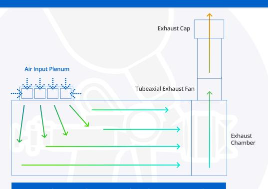
Provides Vertical & Horizontal Air Flow Front to Back
